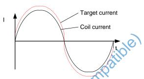
Coil current does not have optimum shape
