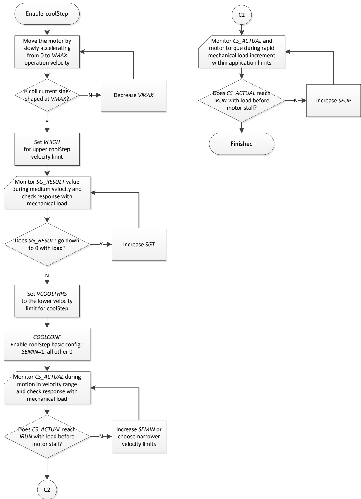
Figure 18.4 Enabling CoolStep (only in combination with SpreadCycle)
