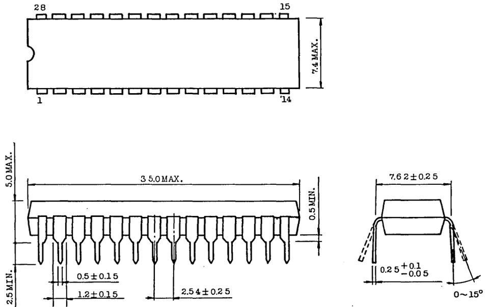
Note: Lead pitch is 2.54 and tolerance is ±0.25 against theoretical center of each lead that is obtained on the basis of No.1 and No.28 leads.
