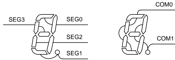
Figure 3.14.9 An Example of Connection of COM and SEG Pins
