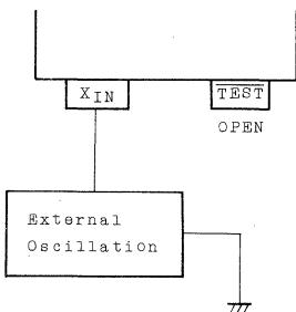
The basic clock of TMP4310APL/TMP4310APLL can be supplied from the external oscillation circuit as shown in the left figure.
