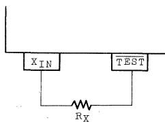
The basic clock of TMP4310APL/TMP4310APLL can be obtained by connecting the resistance as shown in the left figure.
