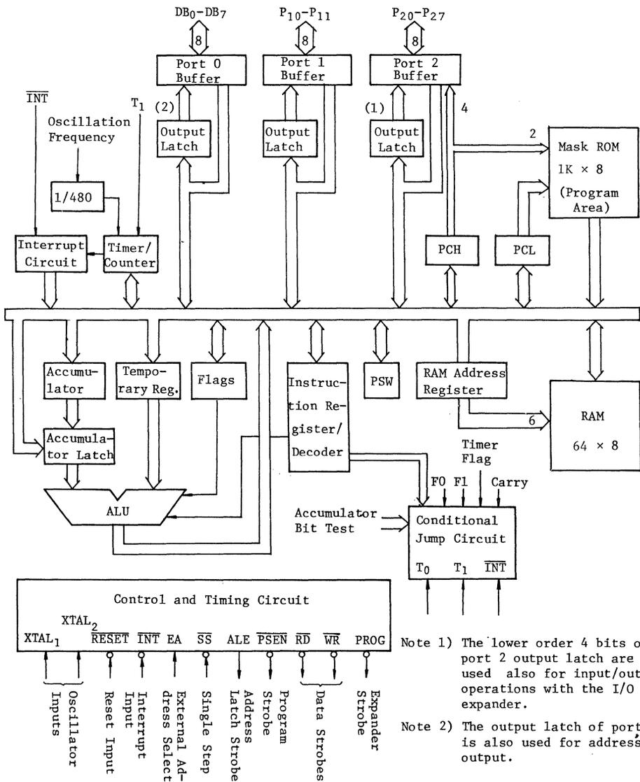
Note 1) The lower order 4 bits of port 2 output latch are used also for input/output operations with the I/O expander.
