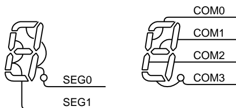
Figure 15-6 Example of COM, SEG Pin Connection (1/4 Duty)
