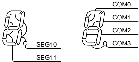
Figure 15-5 Example of COM, SEG Pin Connection (1/4 duty)
