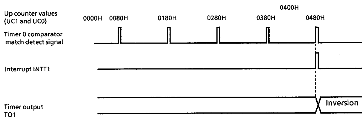
Figure 3.14 (4) Timing Chart for 16-bit Timer Mode
