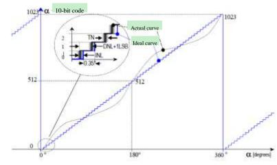
Integral non-linearity (INL) is the maximum difference between the actual position and the measured position.
