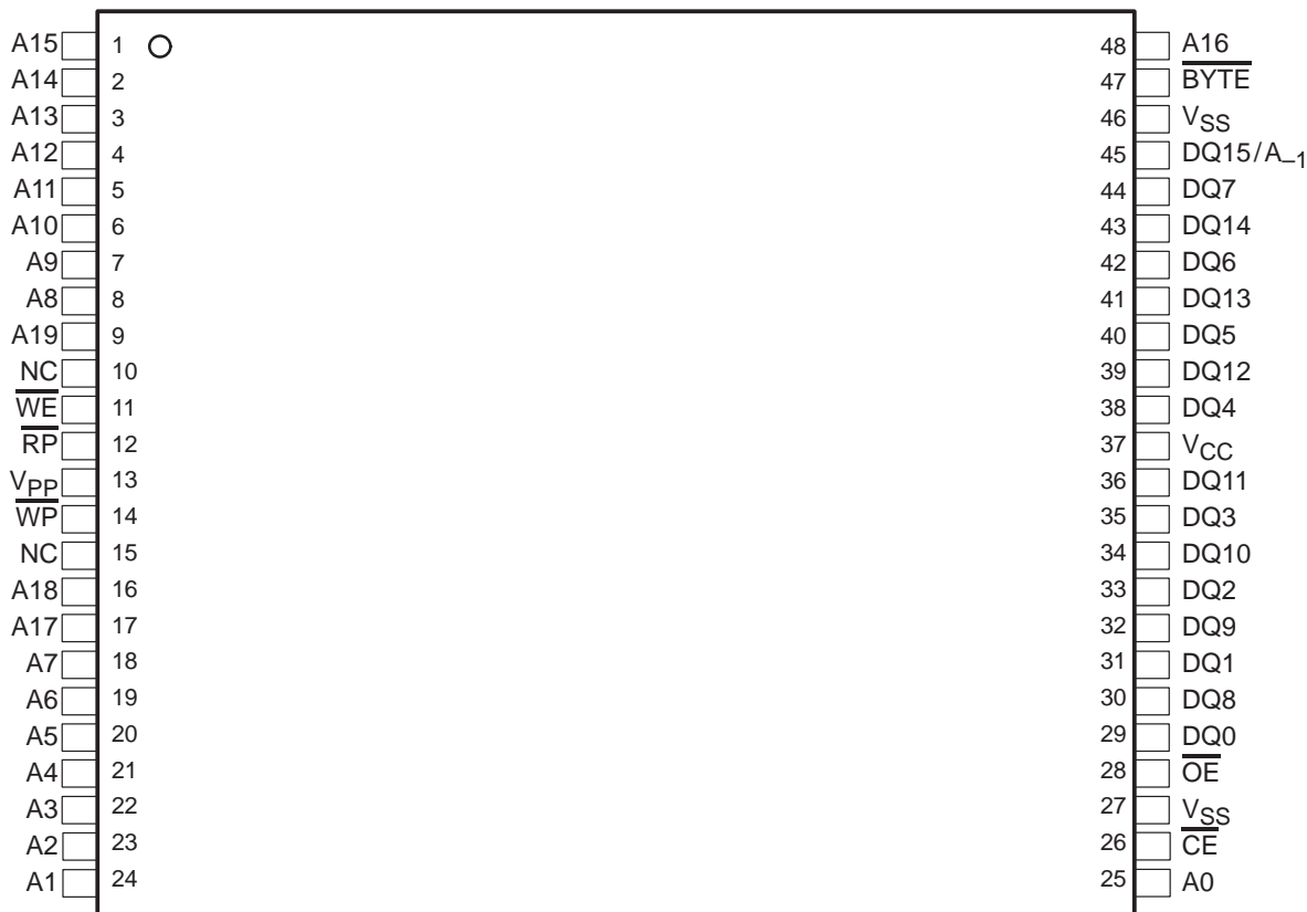
TMS28F1600T/B 48-PIN TSOP (DCD) (TOP VIEW)
