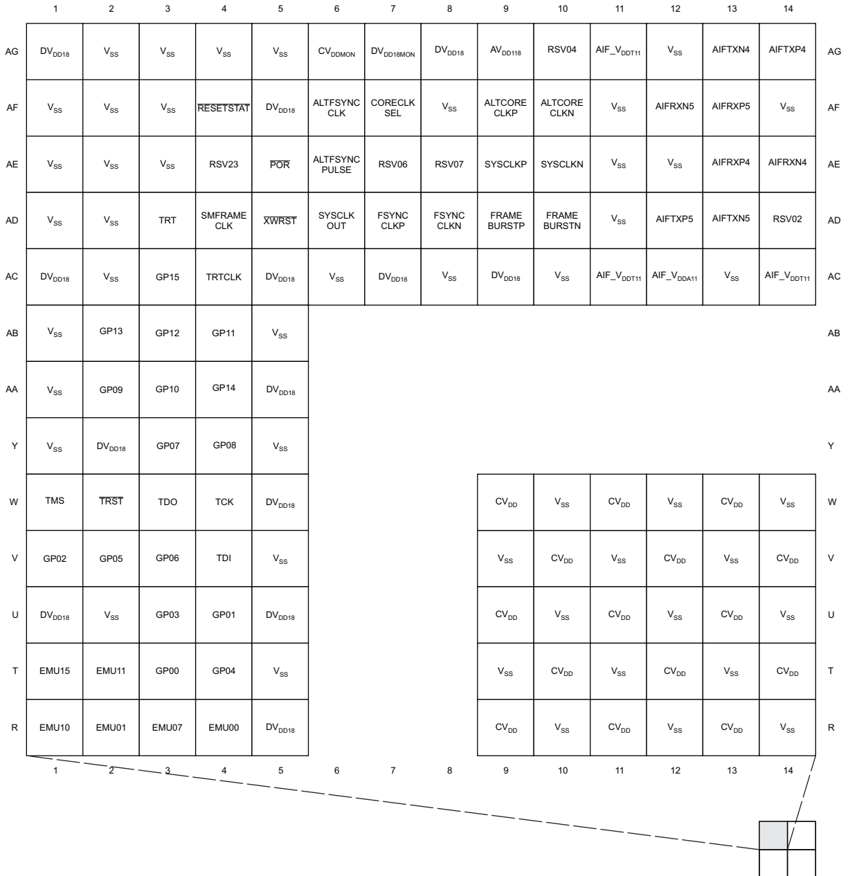
Figure 2-2. TCI6487/8 Pin Map (Bottom View) [Quadrant A]
