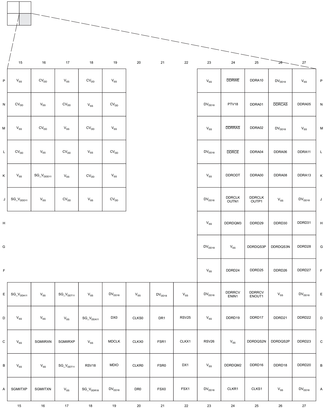
Figure 2-4. TC16489 Pin Map (Bottom View) [Quadrant C]
