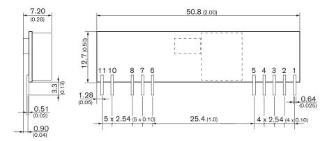
Dimensions in mm (inch) Tolerances x.x  $\pm 0.5$  (x.xx  $\pm 0.02$ ) Tolerances x.xx  $\pm 0.25$  (x.xxx  $\pm 0.01$ ) Pin dimension tolerance  $\pm 0.1$  ( $\pm 0.004$ )
