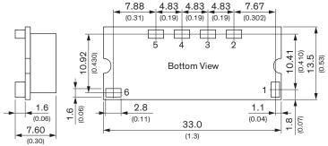
Dimensions in mm (inch) Tolerances x.x  $\pm 0.5$  (x.xx  $\pm 0.02$ ) Tolerances x.xx  $\pm 0.25$  (x.xxx  $\pm 0.01$ ) Pin dimension tolerance  $\pm 0.1$  ( $\pm 0.004$ )
