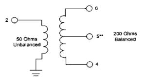
Pins 1 & 3 are grounded to case \*\* Pin 5 to be externally grounded
