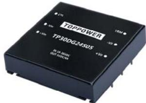
**DESCRIPTION: 30W 1.5KVDC Isolated Wide Voltage Input DC/DC Converters**
