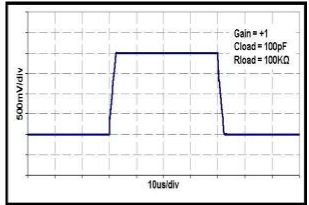
Large-Signal Step Response, 2V Step
