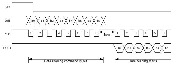
Because the D<sub>OUT</sub> pin is an N-ch open-drain output pin, be sure to connect an external pull-up resistor to this pin (1kΩ to 10 kΩ).
