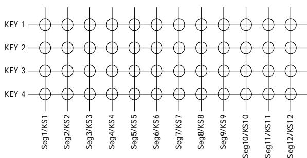
The data of each Key is stored as illustrated below, and is read by a read command, starting from the least significant bit.
