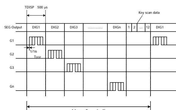
One cycle of key scanning consists of two frames, and data of 12x4 matrices is stored in RAM.
