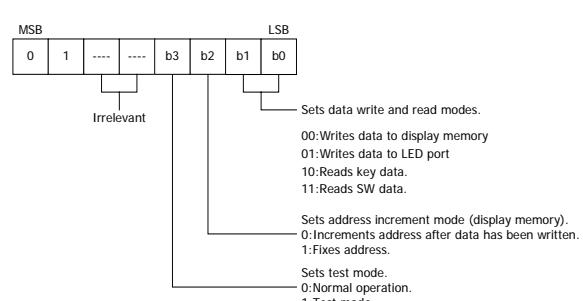
On power application, the normal operation mode and address increment mode set.
