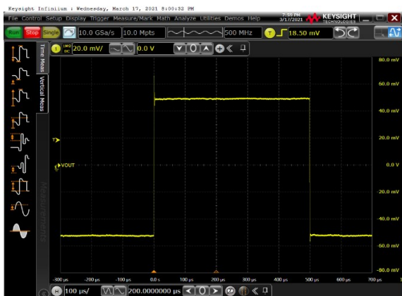
Figure 17. 100-mV Small Signal Step Response
