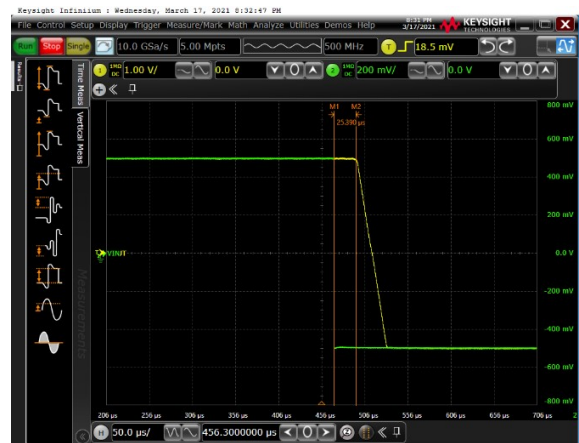
Figure 16. Overload Recovery at Positive Rail
