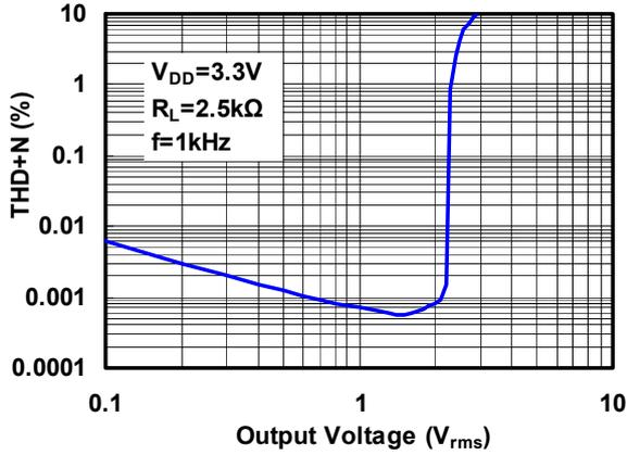
Total Harmonic Distortion + Noise vs. Output Voltage
