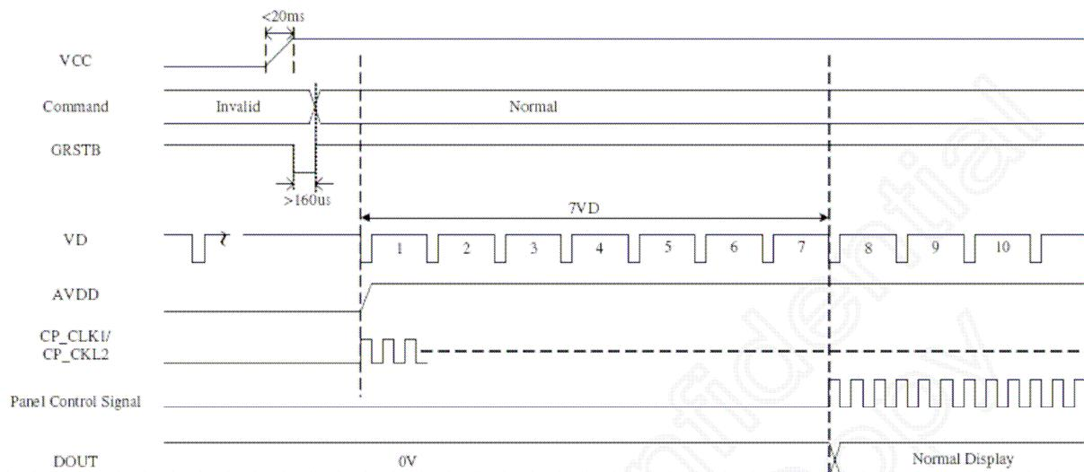
Note 1: After VCC rising, SPI (3-wire) command must wait 160us to start and accomplish all setting of the register value during 7VD field.
