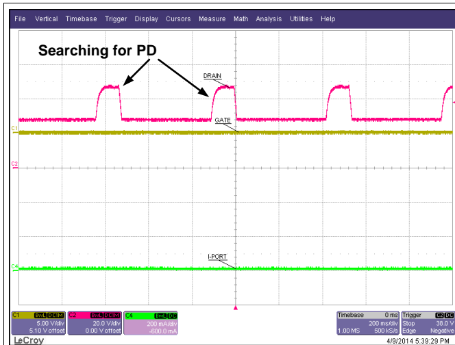
Figure 51. Open Circuit Detection
