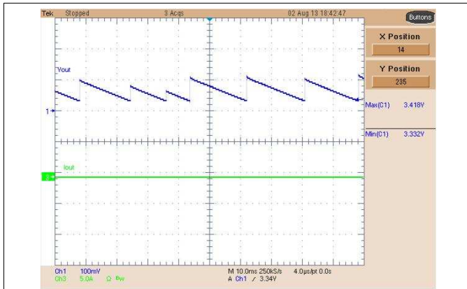
Figure 69. Buck 3 Low-Power Output, No Load
