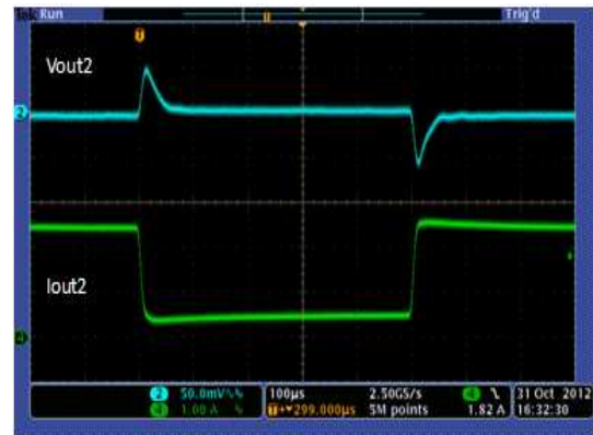
Figure 25. Load Transient, Buck 2 (0.5 A - 2.5 A)
