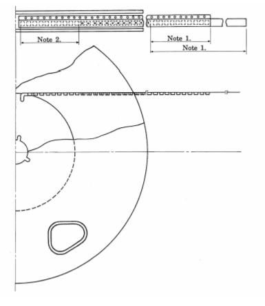
Note 1 : The leader portion shell consist of cover tape minimum length of 300 mm and a piece of carrier tape with empty portion of 100 mm minimum.
