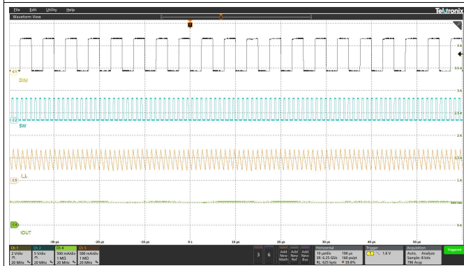
Figure 55. LED Analog Dimming at 99% Duty Cycle and 20 kHz
