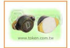
Magnetically Shielded Construction to avoid radiation, Token (TPSDBL) features high breakdown voltage, and very low direct current resistance (DCR). The height only 2.92 mm, they have a footprint of (6.6 x 4.45 mm).
