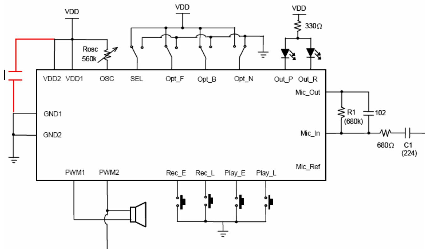
\* R1 is used to control the gain of OP-Amp. A bigger R1 value will lead to larger voice volume. (470K~820K $\Omega$ )
