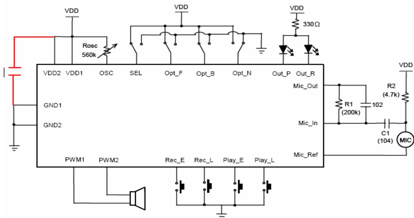
\* R1 is used to control the gain of OP-Amp. A bigger R1 value will lead to larger voice volume. (100K~300K $\Omega$ )
