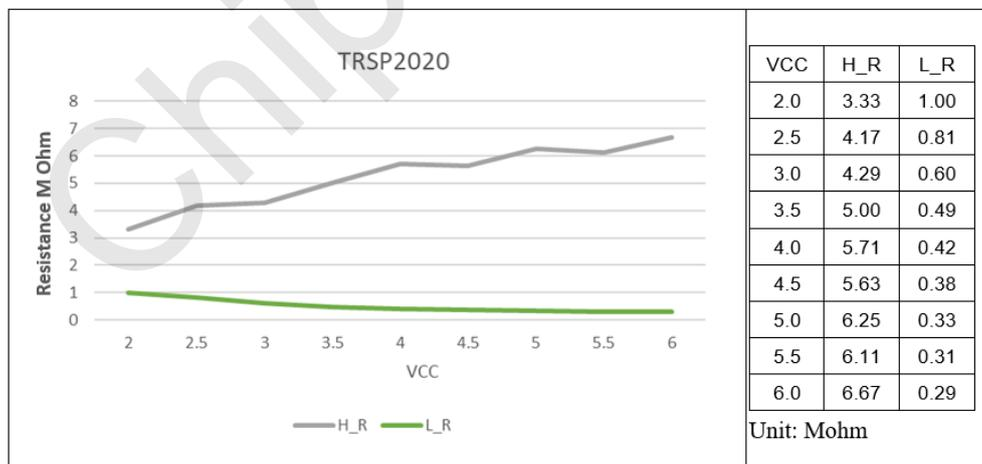
Figure 5 Pull down resistance vs VCC
