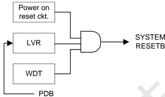
Figure 4 Reset structure
