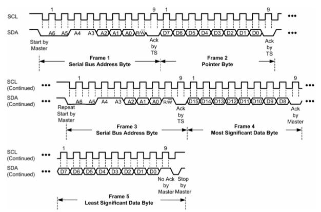
SMBus/I<sup>2</sup>C write to the Configuration Register to Enable Shutdown ((SHDN) <0000 0001 0000 0000>b
