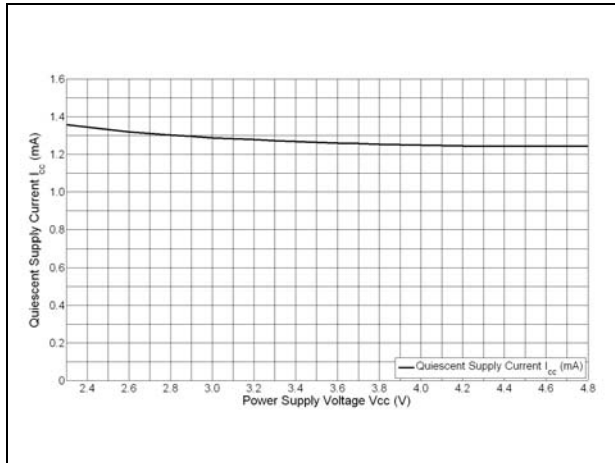
Figure 2. Current consumption vs. power supply voltage
