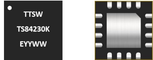
Figure 1 Device Image (16 Pin 3×3×0.8mm QFN Package)
