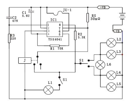
If use JU-1 as shunt detector, the use of capacitor C2 is not necessary. Short circuit detection is used, Pin6 must be open
