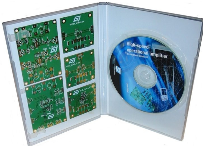
Figure 25: Evaluation kit for high-speed op-amps
