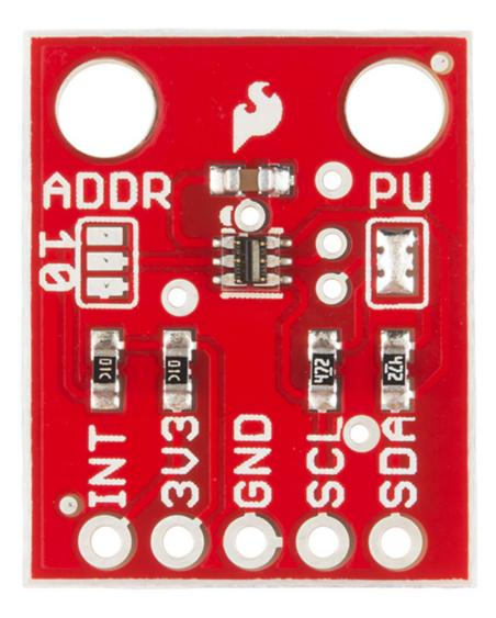
Breakout boards "break out" or connect the tinier pins on tiny components to larger connection points that we humans can deal with. (Robots are welcome to deal with the parts directly.) Breakout boards will also often include support components like resistors and capacitors that make the boards easier to use.
