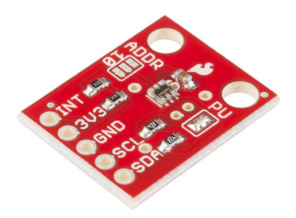
The <u>TSL2561</u> is an inexpensive but sophisticated light sensor. Unlike simpler sensors like <u>photoresistors</u> and photodiodes, the TSL2561 incorporates both infrared and visible light sensors to better approximate the response of the human eye. Because the TSL2561 is an integrating sensor (it soaks up light for a predetermined amount of time), it is capable of measuring both very small and very large amounts of light.
