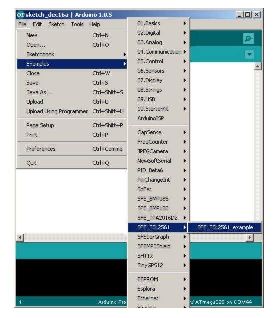
When the example opens, upload it to your Arduino and open the Serial Monitor to 9600 baud. You should see some diagnostic information (if it can't find the device, double check your hardware connections) followed by raw data and lux readings. (See the first page of this tutorial for information on lux.)
