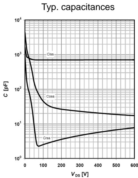
$$C=f(V_{DS}); V_{GS}=0 \text{ V}; f=1 \text{ MHz}$$
