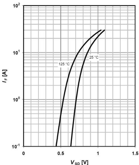
$$I_F=f(V_{SD}); \text{ parameter: } T_j$$
