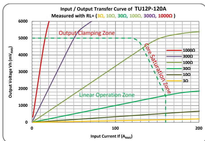
The following figure shows accuracy curve tested with different load resistors. Choosing a high resistance value will give high sensitivity, but the core saturation begins at lower input current also. In the case of a 300Ω load, the secondary voltage clamping occurs at 50ARMS input because of the output is 5VRMS which have a peak at 7.07V
