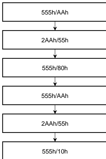
Auto Chip Erase Command Sequence (address/data)
