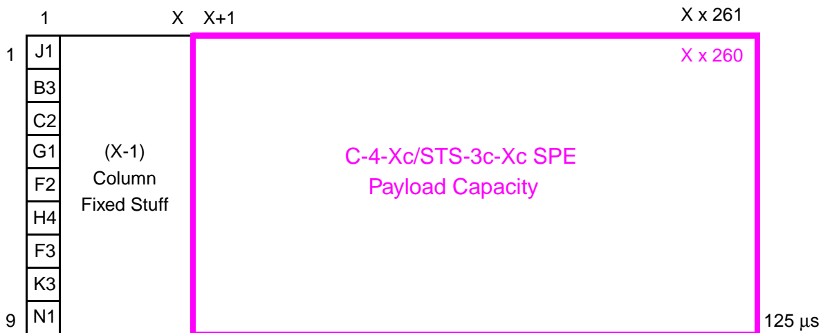
Figure 5. VC-4-Xc/STS-Nc (N = 3X) Contiguous Concatenation Structure for SONET/SDH
