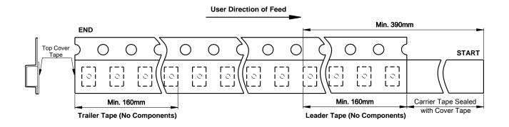
**Note:** There shall be a leader of at least 230mm which may consist of carrier tape and/or cover tape or a start tape followed by at least 160mm of empty carrier tape sealed with cover tape.
