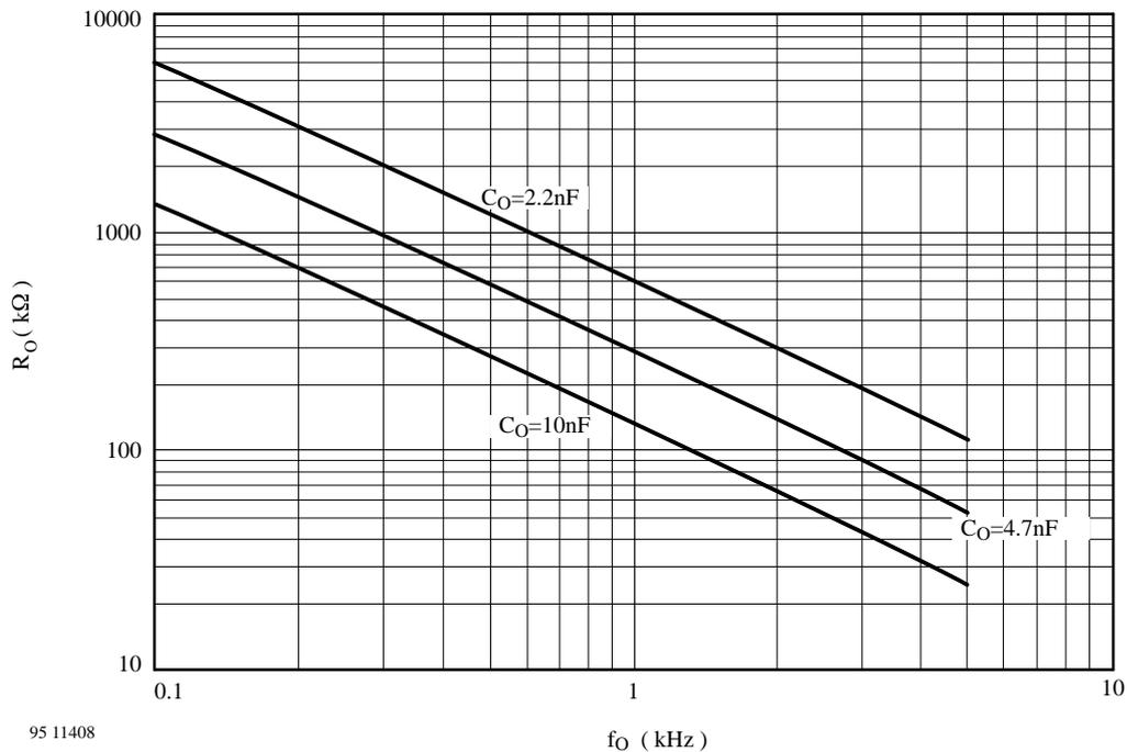
Figure 9. Frequency versus resistance for different capacitance values
