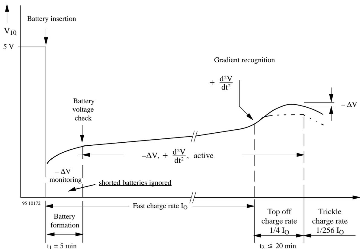
Figure 3. Charge function diagram,  $f_{osc} = 800 \text{ Hz}$
