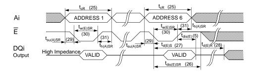
Software Controlled STORE/RECALL Cycle<sup>x, y, z, aa</sup> ( $\overline{E}$  = LOW after STORE initiation)
