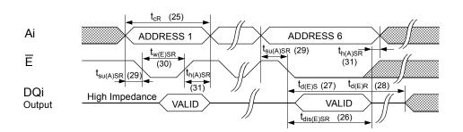
t: W must be HIGH when E is LOW during the address sequence in order to initiate a nonvolatile cycle. G may be either HIGH or LOW throughout. Addresses 1 through 6 are found in the mode selection table. Address 6 determines wheter the U631H256XS performs a STORE or RECALL.
