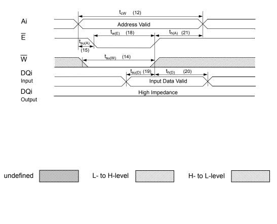
i: If  $\overline{W}$  is low and when  $\overline{E}$  goes low, the outputs remain in the high impedance state.
