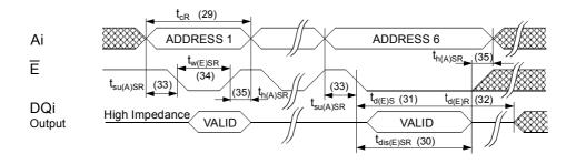
u: W must be HIGH when E is LOW during the address sequence in order to initiate a nonvolatile cycle. G may be either HIGH or LOW throughout. Addresses 1 through 6 are found in the mode selection table. Address 6 determines wheter the U63716 performs a STORE or RECALL.
