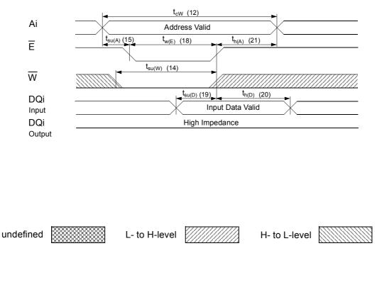
If  $\overline{W}$  is low and when  $\overline{E}$  goes low, the outputs remain in the high impedance state.  $\overline{E}$  or  $\overline{W}$  must be V<sub>IH</sub> during address transition. i:
