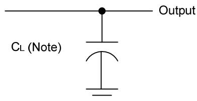
Note:  $C_L$  includes probe and jig capacitance.
