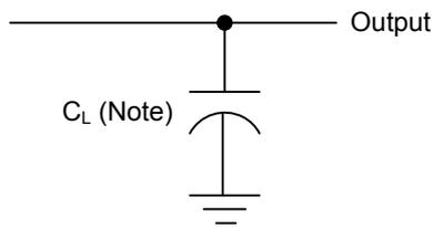
Note:  $C_L$  includes probe and jig capacitance.
