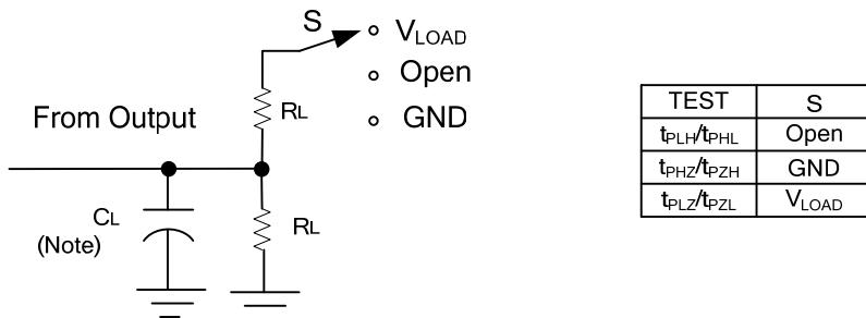
Note:  $C_L$  includes probe and jig capacitance.
