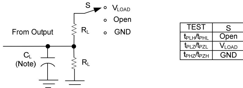
Note:  $C_L$  includes probe and jig capacitance.
