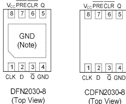
Note: Connect exposed pad to GND.
